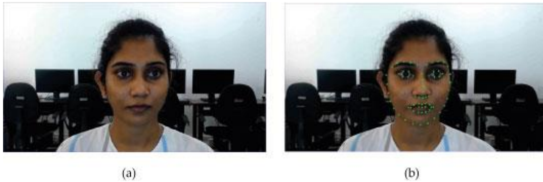
Figure 2. (a) Input face image to the algorithm, (b) Dlib 68 face landmark detector
