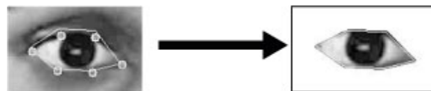
Figure 3. Generating left eye mask using 36-41 Dlib facial landmarks; left: left eye with eye landmarks, right: left eye mask
