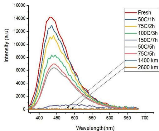
**Figure 4:** Different Fluorescence spectra obtained for artificially aged and literarily aged Caltex DS 40 engine oil samples.
