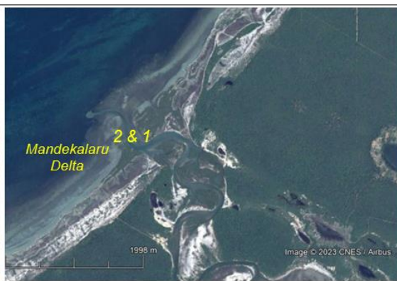
Figure 4.2. Marine entrance of the Mandekal Aru shows the ebb tidal mud flat formation in 2017. 2 & 1 represent the lower and upper entrances (Google Image).
