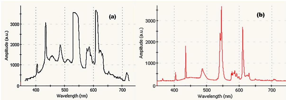
Figure 6. Spectrum of a common CFL lamp emission taken by (a) presented spectrometer (b) ocean optics commercial spectrometer.
