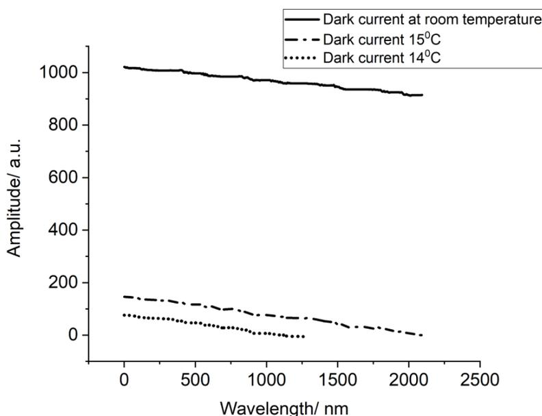
Figure 8. The reduction in dark current with a reduction in the CCD temperature.
