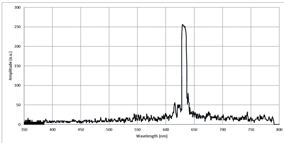
Figure 7. Spectrum of a 630 nm laser diode emission.
