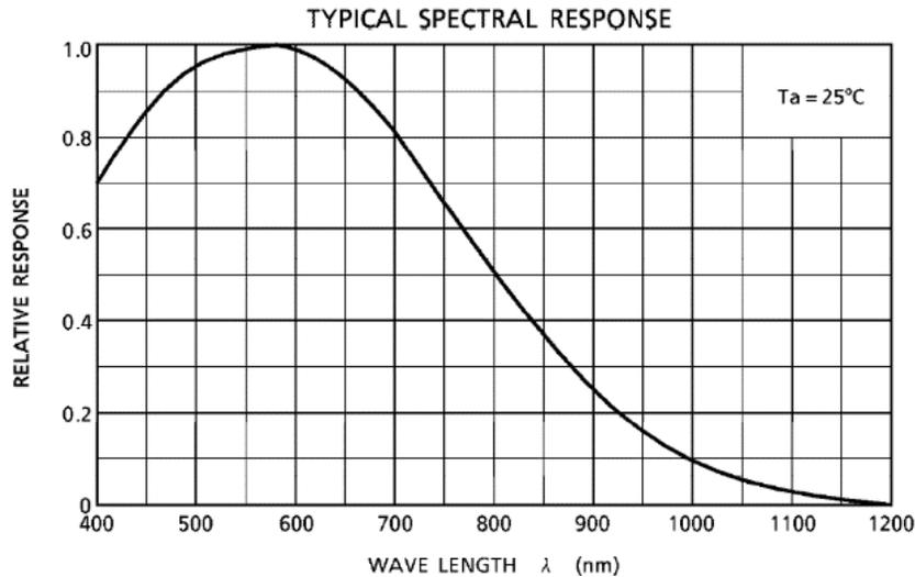
Figure Error! No text of specified style in document.. Wavelength response of TCD1201D linear CCD.
