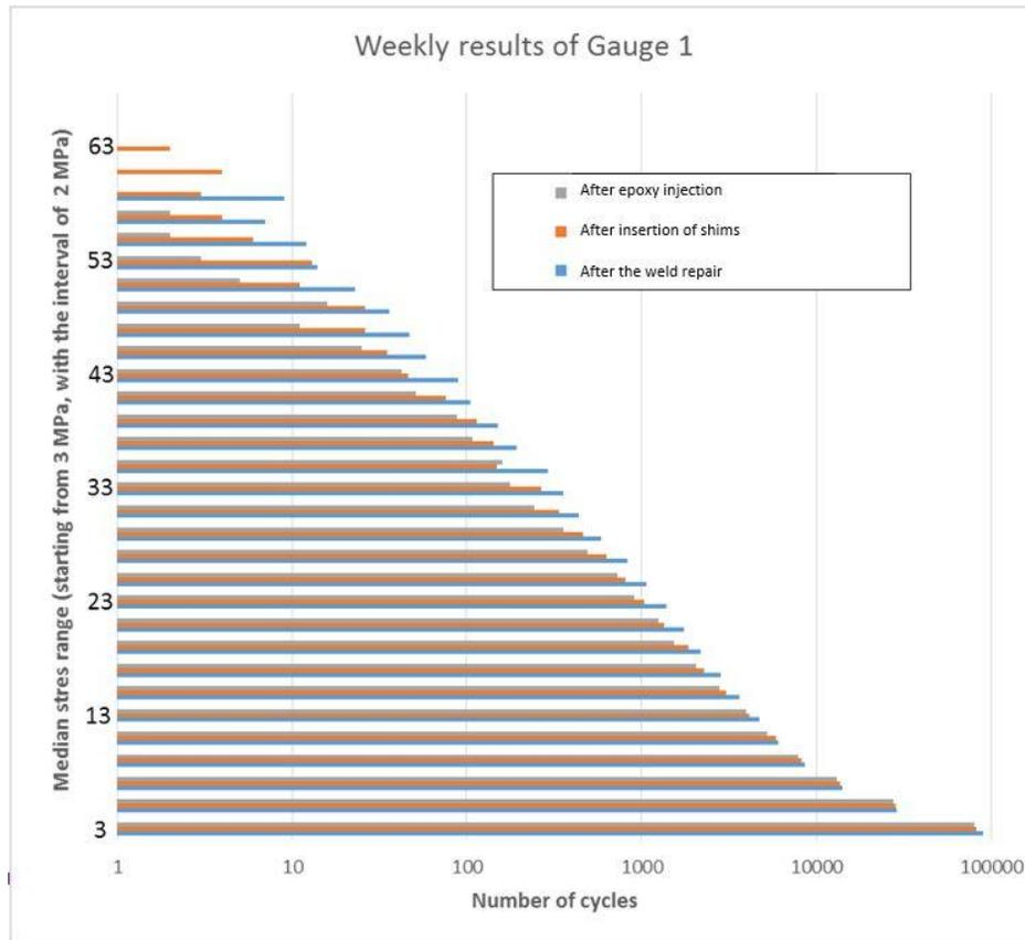
**Figure 4.** Median stress range for after the weld repair, after insertion of shims and after epoxy injection for Gauge 1.
