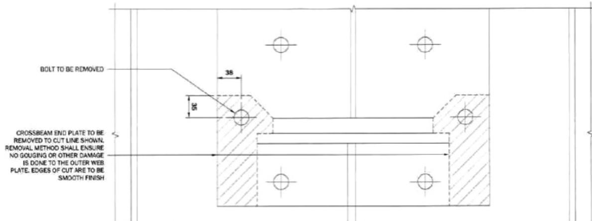
**Figure 1.** Engineering drawing of the end plate with instructions on how to remove it safely.
