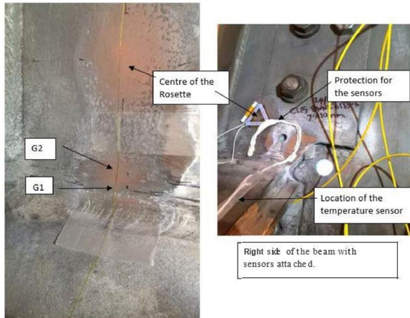
Figure 3. Placement of G1, G2, temperature sensor and a rosette on the end plate.
