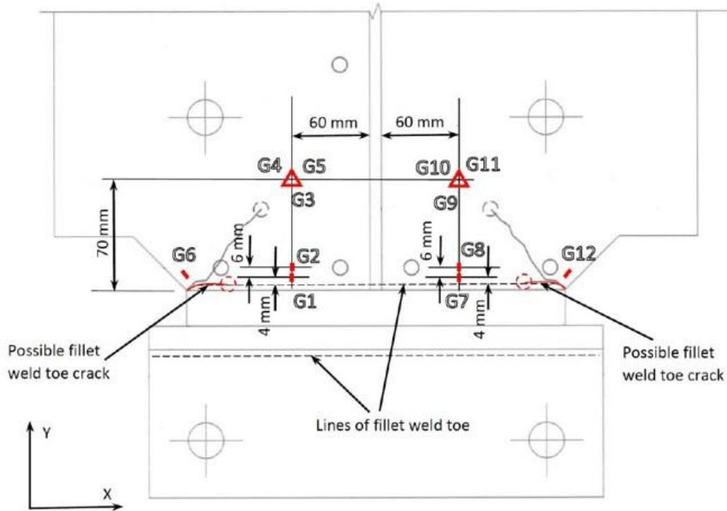
**Figure 2.** Detailed engineering drawing showing the placement of twelve FBG sensors.
