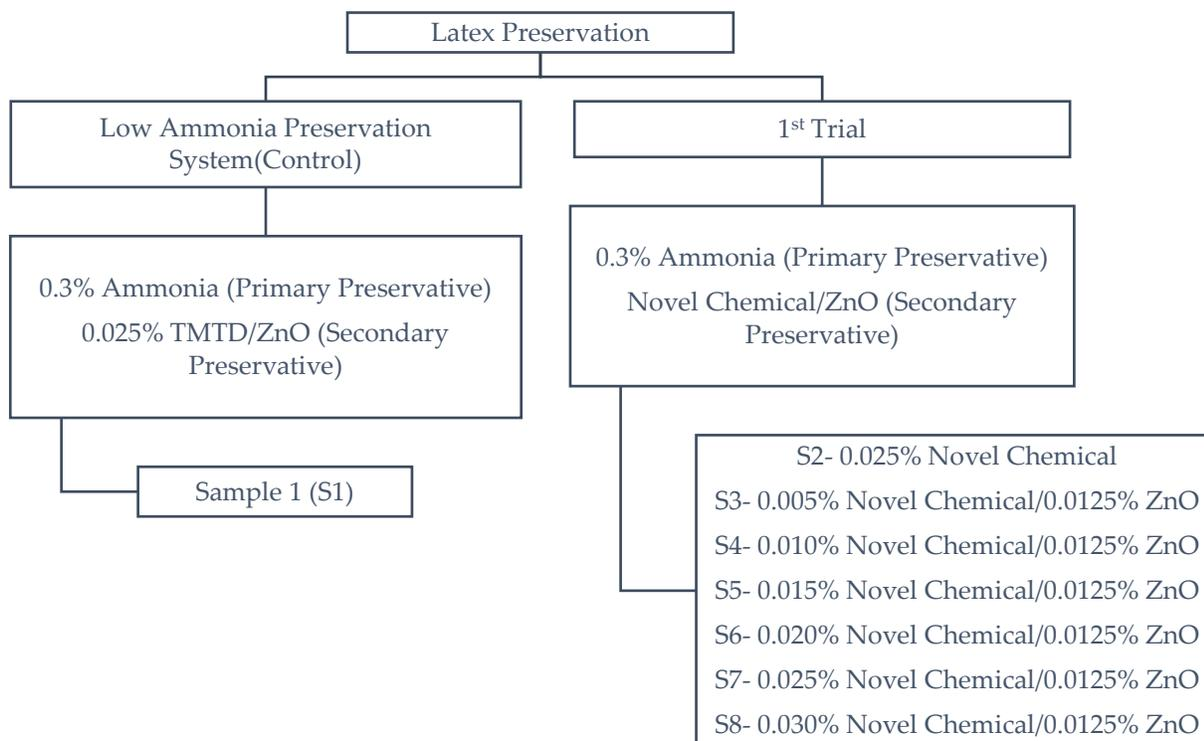
**Figure 1-** Schematic diagram of trial 1
