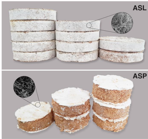
Fig. 1. Image showing Mycelium plates made from different fungal strains: ASL- L. squarrosulus with Albizia sawdust, ASP- P. ostreatus with Albizia sawdust
