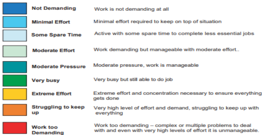
Figure 2: IWS for rail signallers (color codes run from blue for not demanding to red for work is too demanding)
