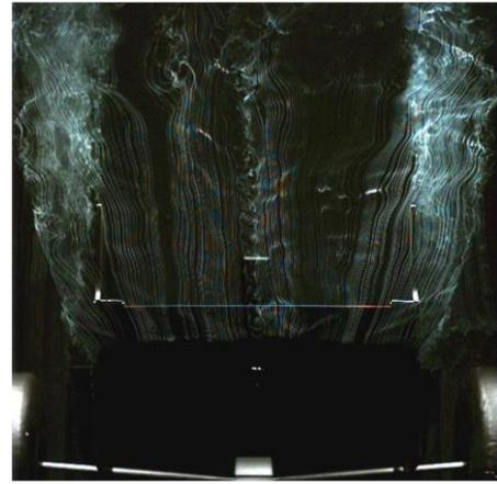
Fig. 3. Smoke visualisation over the rear wing for the design case, vertical elevation with flow moving from bottom to top [20].
