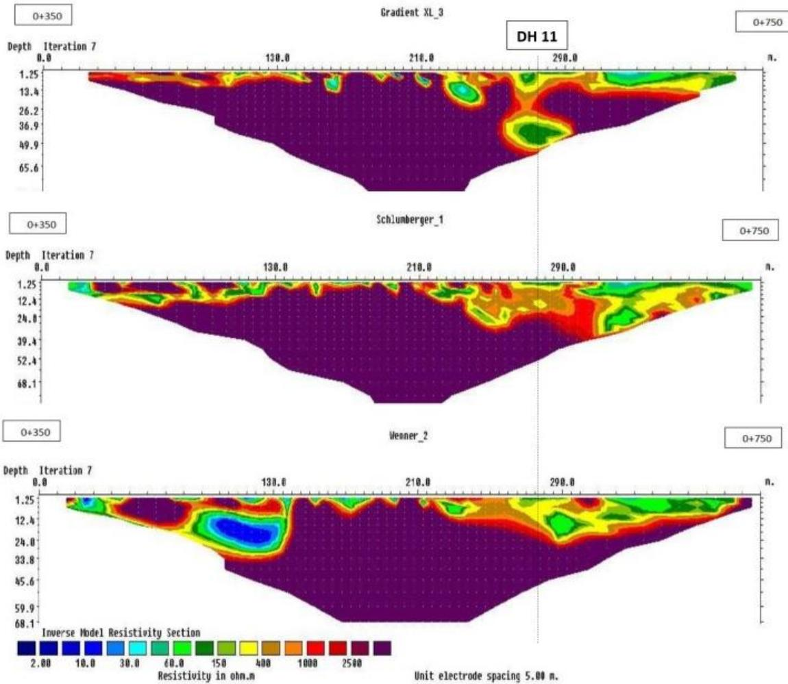
Fig. 10. Locations of DH 11 in ERT 3 using Gradient XL, Schlumberger & Wenner methods
