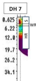
Fig. 13. Comparison of borehole data with ERT results in ERT 4
