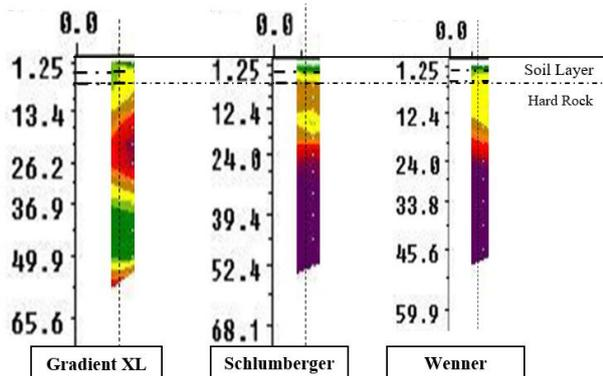
Fig. 14. Comparison of borehole data (DH11) with ERT results in ERT 3
