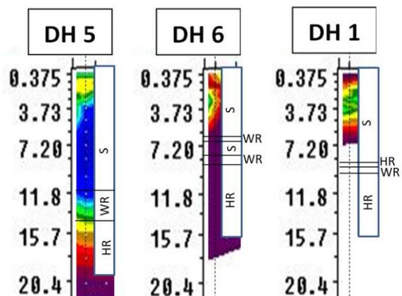
Fig. 11. Comparison of borehole data with ERT results in ERT1
