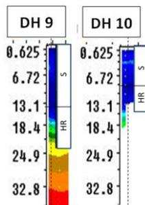
Fig. 12. Comparison of borehole data with ERT results in ERT2
