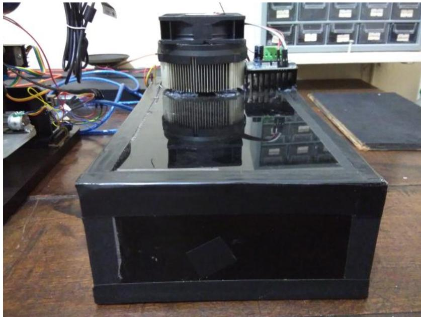
Figure 4. The custom-built spectrometer.
