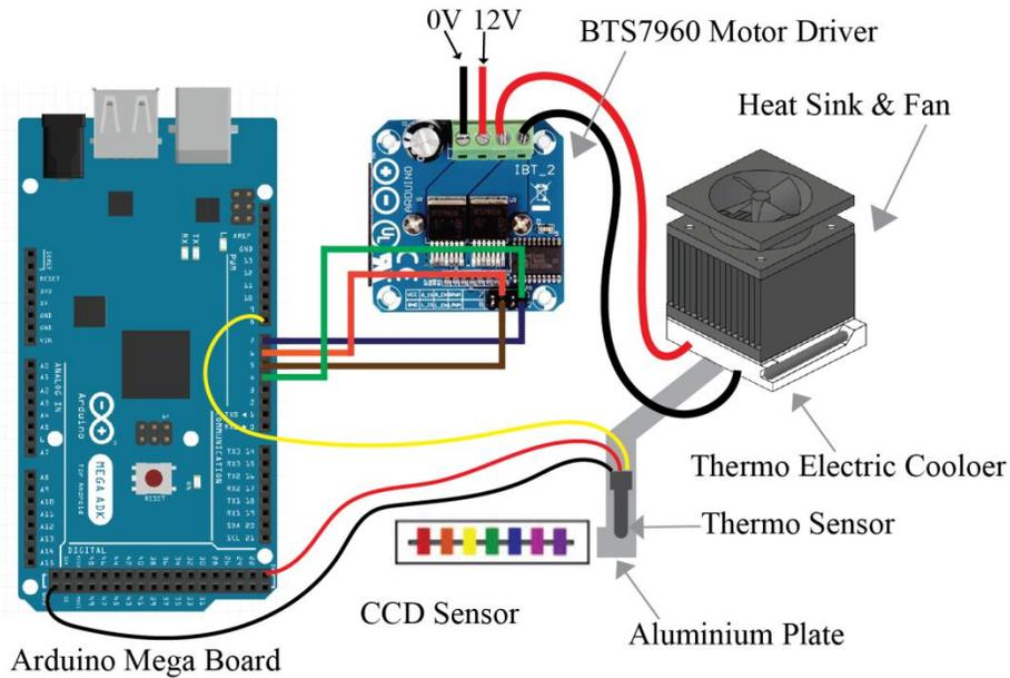
Figure 3. Circuit diagram and configuration of the cooling system.
