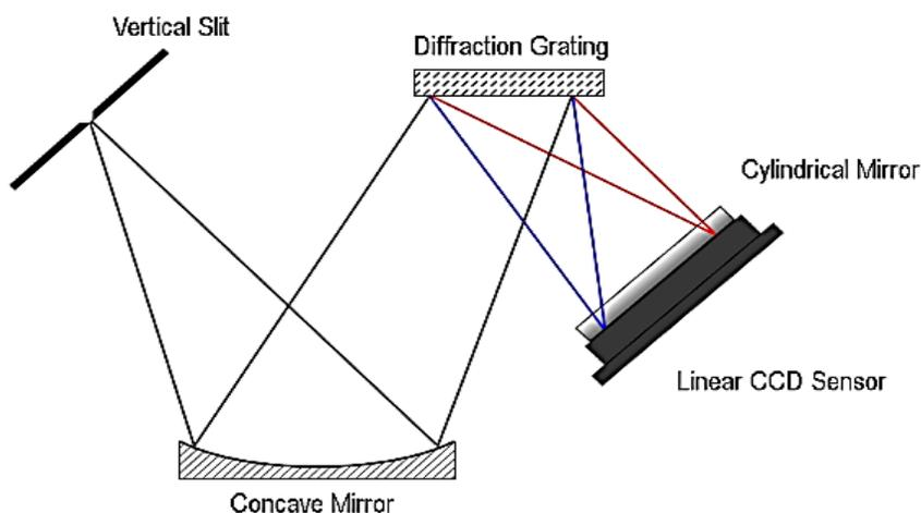
Figure 1. Component arrangement of the optical setup of the spectrometer.
