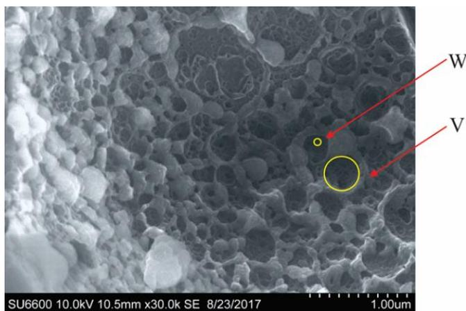
Figure 13. SEM image VMRH in  $\mu\text{m}$  scale (V-Void and W-Window).
