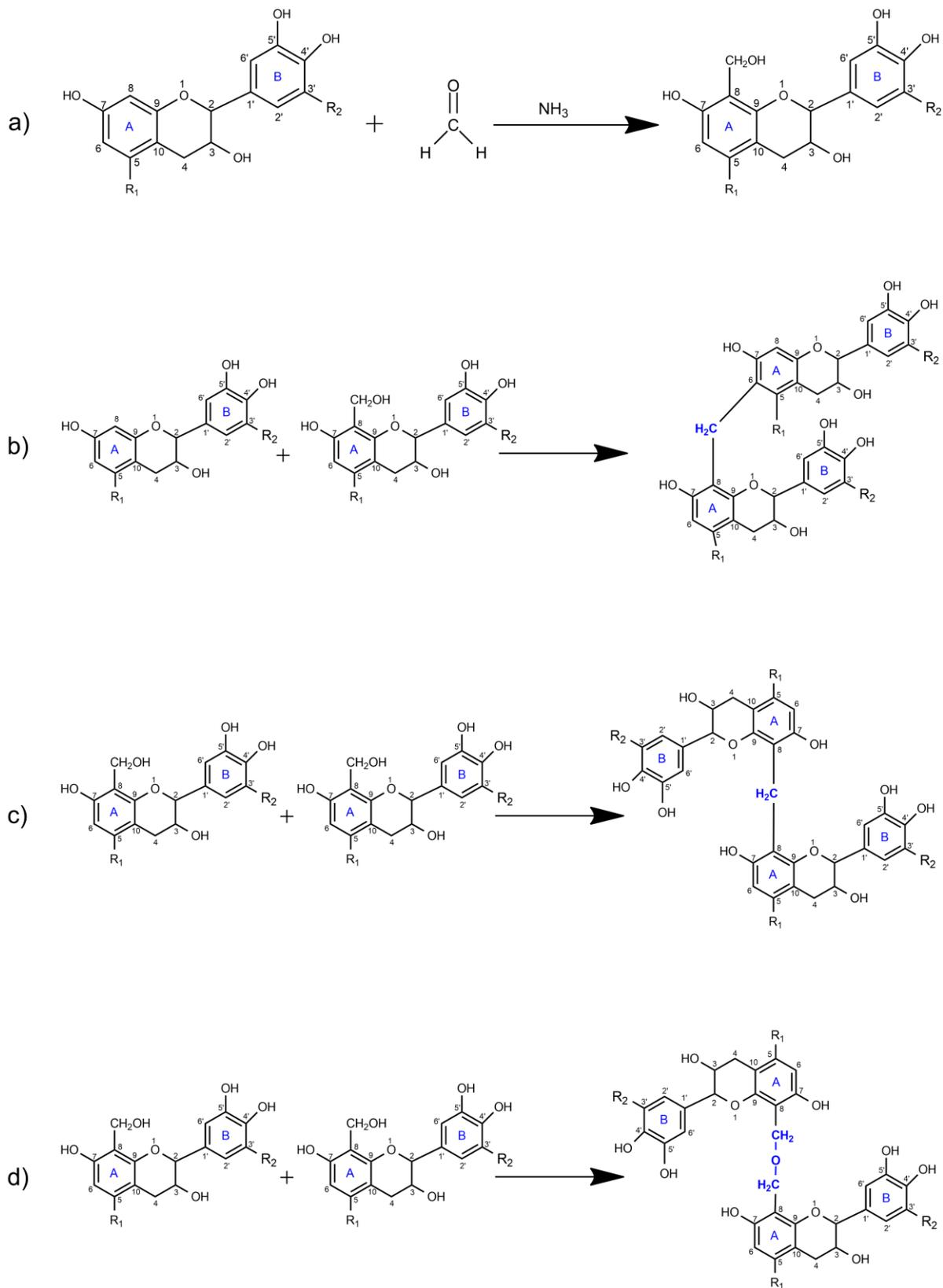
Figure 2. Reaction of condensed tannin with formaldehyde.
