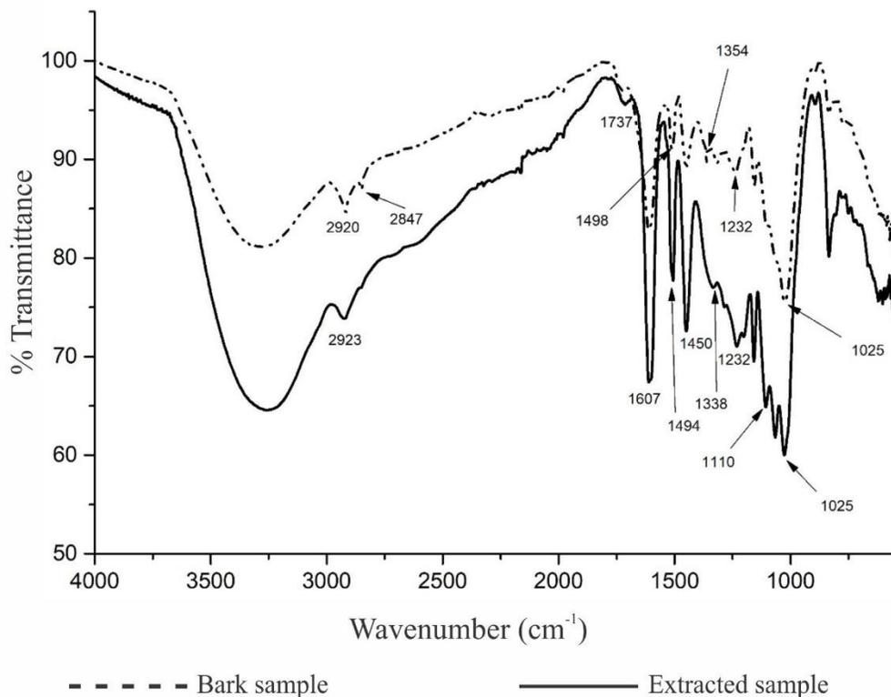
Figure 7. FTIR Spectra of bark sample and extracted taninns.
