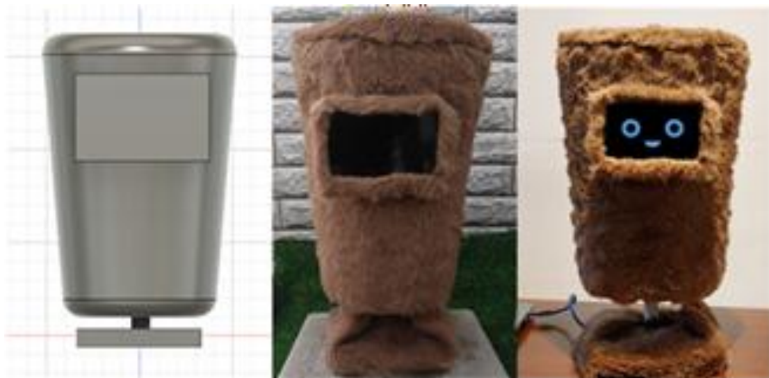
Figure 4. Left: 3D design of the robot created by Fusion 360, Middle: Final design of the robot, Right: Physical appearance of the robot with emotions
